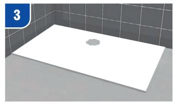
Ensure DEC fits neatly into the recess. Mark shower trap position.
