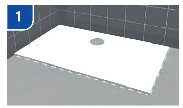
Locate DEC in the corner to which it is going to be finally positioned and mark lines around the outer edge.
