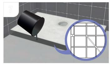
Square ribbed underside allows DEC to settle on a cement or screed base eliminating slippage during installation. Carefully place DEC into position. Check levels in both directions, gently tap DEC down until level on all 4 sides. It may be necessary to add more sand and cement, do this by slightly lifting the DEC and adding in the mixture. Gently tap again until level on all 4 sides.
