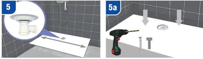
**METHOD 1 (as shown in points 5 & 5a)** - Set the trap body into the floor. Place the trap flange into the DEC ensuring it finishes flush with, or just below the surface on which the sheet flooring is to be laid. Secure flange to the DEC, there are a number off countersunk indentations in the flange to assist with this. Connect trap to waste pipe for outflow drain.
